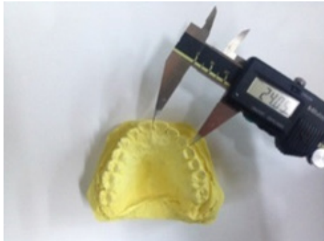
Figure 4: Measurement of anterior arch length with Mitutoyo Digimatic Caliper
