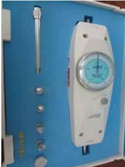
Fig. 7. Handy Analog Push-Pull Gauge
